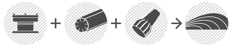
The length of the throw determines the area being irrigated. A longer throw increases the area covered by the irrigation with the effect of making the irrigation more cost effective. At the same time a longer throw determines also a reduction of the instantaneous water application rate thus improving the water take-in of the soil.
