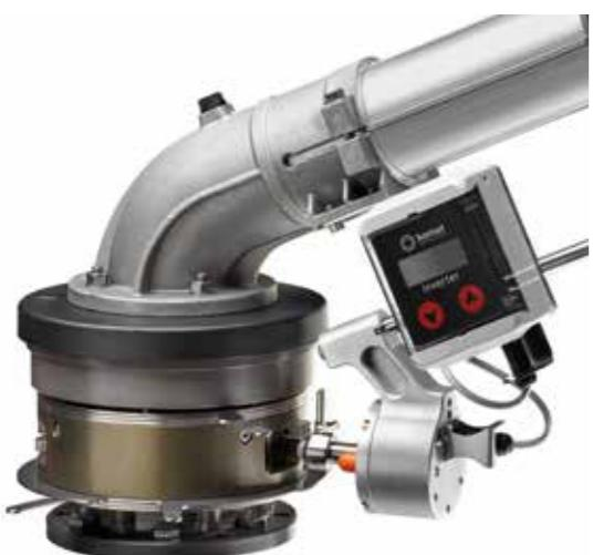
The patented Komet Inverter used on travellers, is a time-controlled device to change irrigation sectors while operating. It allows to irrigate two completely independent irrigation sectors which need to be set before starting operation. Starting in the first irrigation sector, the big volume gun will change automatically into the second irrigation sector after a pre-set time has elapsed. If a subsequent full-circle operation is required, a full-circle adapter is available.
