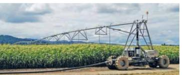
The cart is built to pull. It is capable of handling up to an 8" hose depending on flow requirements.
